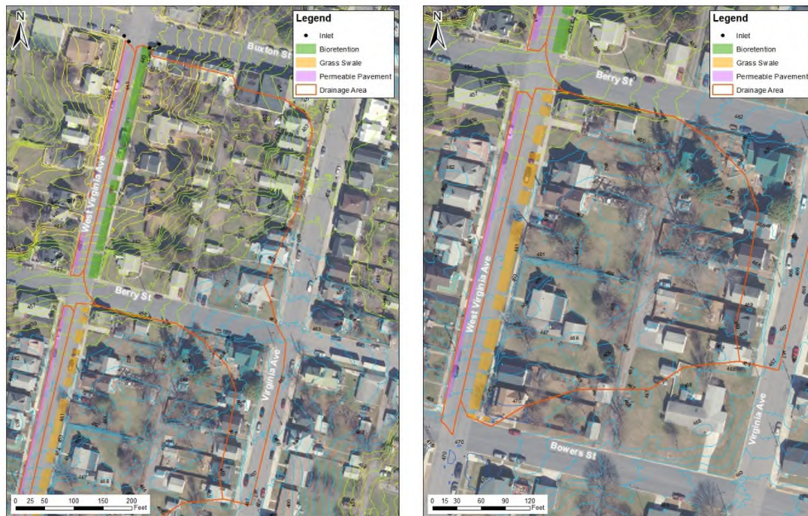
Figure 16. Drainage areas for the northern bioretention and permeable pavement (left) and southern grass swale and permeable pavement (right) on West Virginia Avenue.
